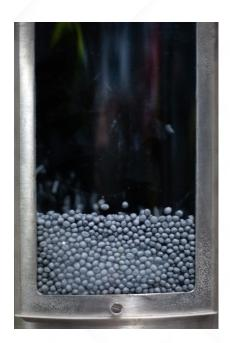
Expanded polystyrene (EPS) is manufactured from expandable polystyrene beads. These beads are produced by polymerising Styrene Monomer and adding pentane as an expansion agent along with a flame-retardant additive to produce a flame-retardant grade where required.
