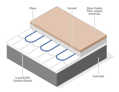
Board 2: A 800 x 300mm board with radius grooved return slots at 200mm centres to suit 16, 20 and 22mm diameter pipes.
