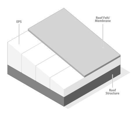
A main consideration for a specifier is to decide which weather proof finish is required and then build up a compatible system to accommodate this, coupled with the need to take into account the effect of heat on the construction both during construction and after completion.
