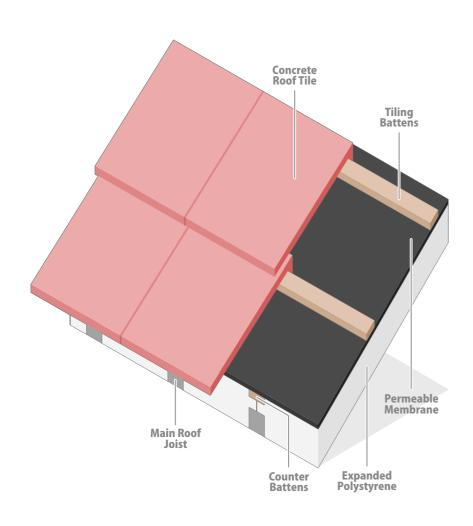
S and B EPS pitched roof panels are manufactured in various sizes to suit most rafter centres, thicknesses and edge profiles to suit nominal 38 or 50mm rafter centres plus, if required, an edge detail can be produced to accommodate double lapped rafters.
