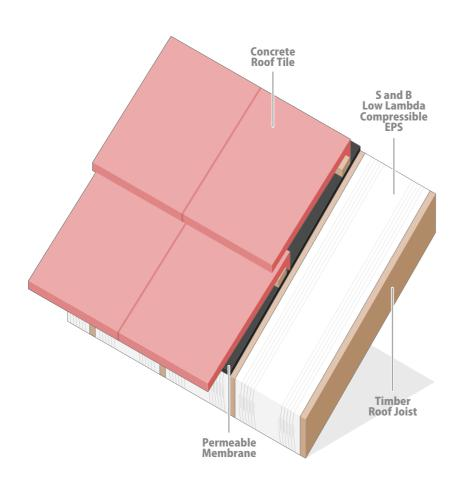
S and B EPS compressible roof panels can accommodate a wide range of rafter centres encountered with the minimum of fuss and greatly reduce the need for on-site cutting as experienced with conventional boards.
