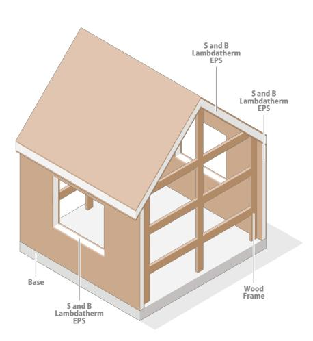
One method of construction that will be at the forefront of this building design and technology is SIPS panels.
